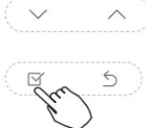
Press the button “ $\downarrow$ ” or “ $\uparrow$ ” to set the time of On timer, and then press the Confirm button to confirm the setting.
