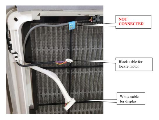
The panel comes with 3 connectors. Only 2 has to be connected
