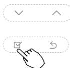
When the air conditioning unit is off, into the query function of temperature, press “ $\vee$ ” or “ $\wedge$ ” to select tyPE. Press “Confirm” into setting state, press “ $\vee$ ” or “ $\wedge$ ” to select the type, then press “Confirm” to complete it.
